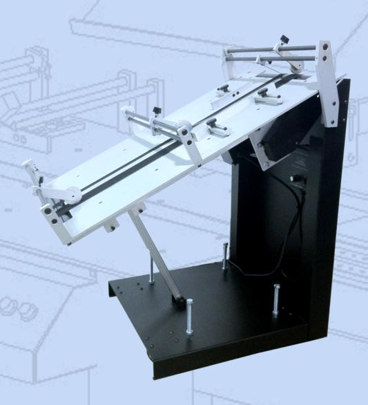
Improve your production capability and bottom line by running the 350INC fully adjustable incline conveyor inline with your existing folder for a seamless one pass operation on all of your inkjet and tabbing applications. The unit is capable of rotating a wide range of product sizes and thicknesses left or right 90 degrees from the original infeed orientation.
